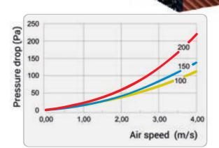
**Note:** There is a risk of droplet falling at an air speed of more than  $3\,\text{m/s}$ .
