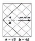
Suitable for application conditions where a good balance between humidification efficiency and pressure drop is required.
